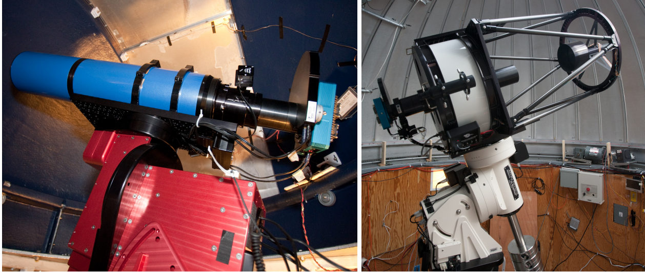
Figure 2. The 5.3 inch f/5.4 VYSOS-5 telescope built by Stellarcue Telescopes (left) in its dome at Mauna Loa Observatory. The 20 inch f/8.2 VYSOS-20 telescope built by RCOS (right).
