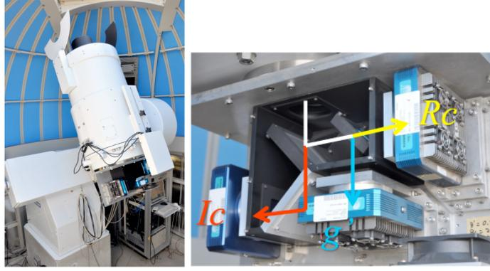
Figure 1. Telescope and camera system of MITSuME Okayama. Left panel is the 0.5m reflector with the simultaneous three-band imager. Right panel is the closeup picture of the three-band imager. This imager, which has a wide field of view ( $26'' \times 26''$ ), enables to take simultaneous images in g', Rc, and Ic bands.
