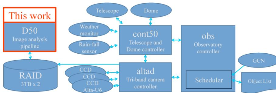
Figure 2. Flowchart for observation and reduction of MITSuME Okayama. This robotic system is mainly controlled by Java based software (cont50 and obs). The CCD camera is managed in altad. The image analysis pipeline D50 is this work.
