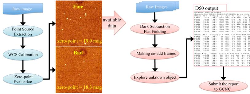
Figure 3. Flowchart of two analysis sequences. Left half and Right half show in real-time parallel processing and about the analysis for GRB afterglow, respectively.
