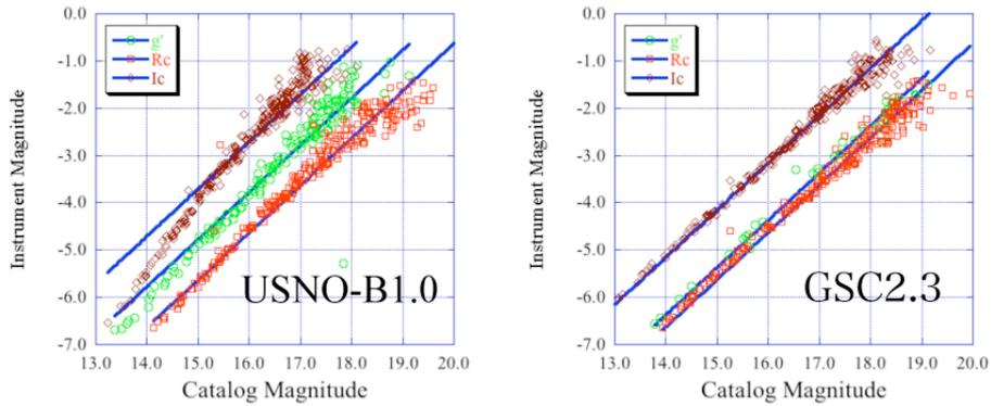
Figure 4. Relation between catalog magnitude and instrumental magnitude. Left panel shows non-linear trends about USNO-B1.0. Right panel is the relation for GSC2.3. The vertical axis is the instrumental magnitude and the horizontal axis is the magnitude from each catalog. Open circles, open squares and open diamonds show the data points for  $g'$ , Rc and Ic, respectively. The solid lines are the fitted lines for the slope of 1.0.
