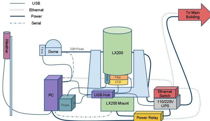
Figure 1. Schematic of our robotic telescope setup.
