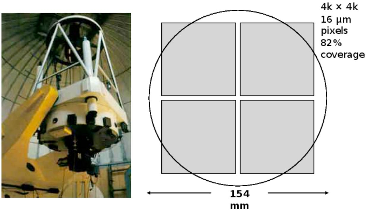
Figure 4. Left panel: USNO 1.3 m telescope, similar to the TAOS II model. Right panel: Possible layout of the TAOS II camera, using a mosaic of four 4k×4k CMOS images with 16  $\mu\text{m}$  pixels.
