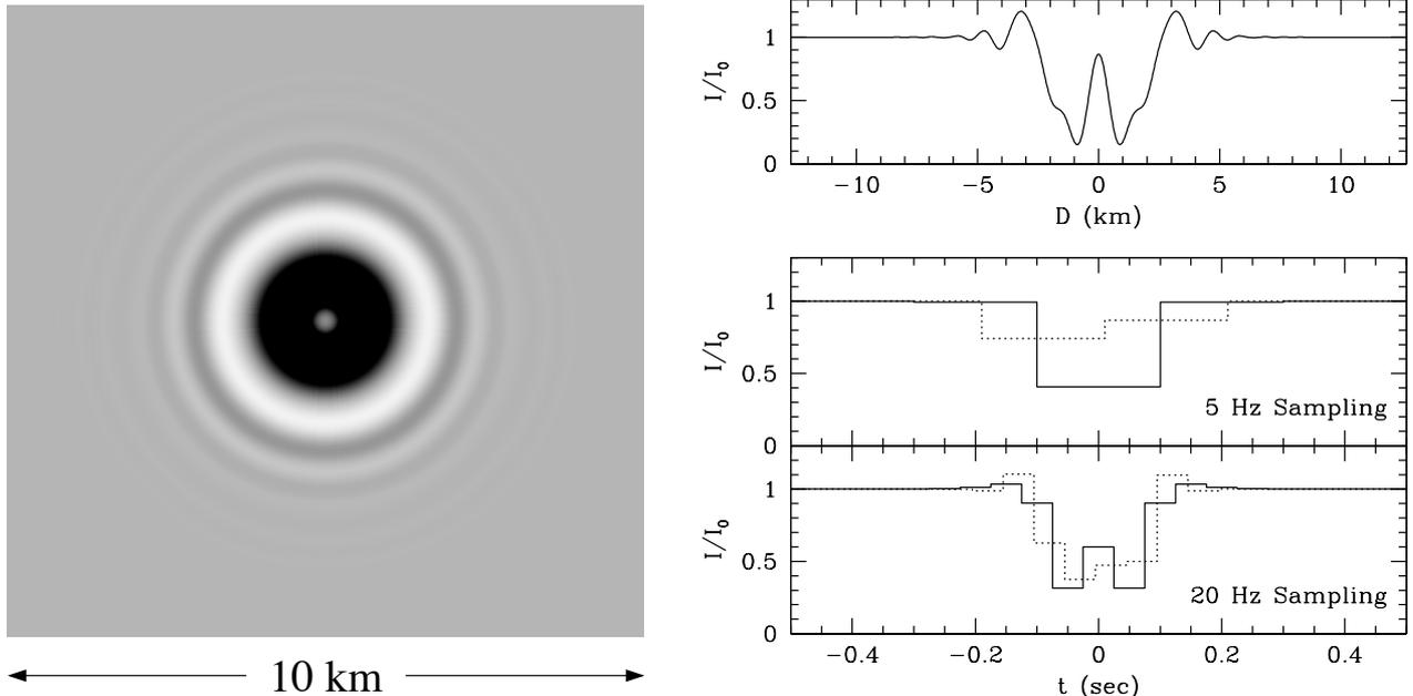
Figure 1. Left panel: diffraction shadow projected onto the surface of the Earth from a 3 km diameter KBO at 43 AU. Right panel top: perfectly sampled lightcurve assuming zero impact parameter. Right panel bottom: same lightcurve as sampled by the TAOS system at 5 Hz and 20 Hz. Solid curves have measurements centered on event, dotted lines shows lightcurves where sampling is out of phase with event.
