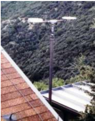
The weather sensors (left) included a rain sensor (left side of pole) and cloud detector (right side of pole). An observatory control computer was added to our wall-mounted lineup of control systems (shown at the right with Lou Boyd).
