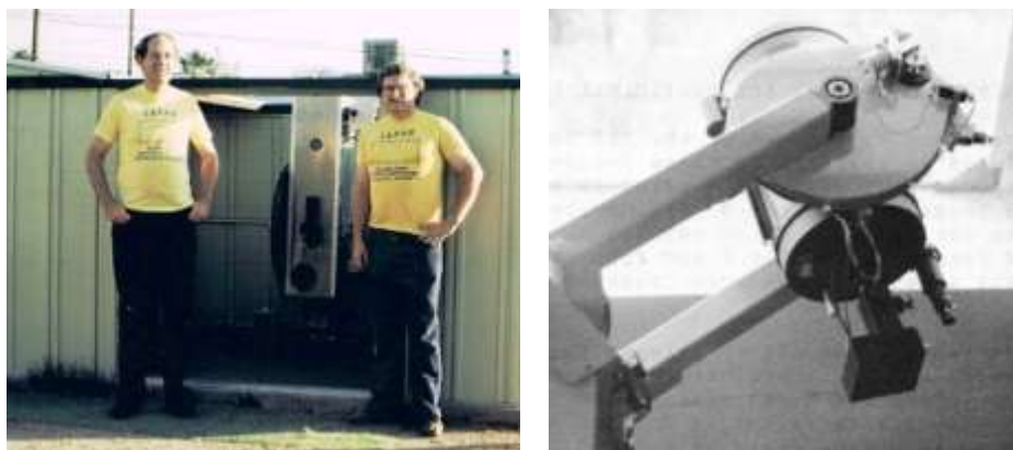
Russ, Lou, and the Phoenix 10 robotic telescope (left) pose before its first full night of automatic operation on October 13, 1983. Russ assembled the Fairborn 10 robotic telescope (right) from a DFM Engineering mount, Meade 10-inch Schmidt Cassegrain optics, and an Optec SSP-4 VRI photometer.
