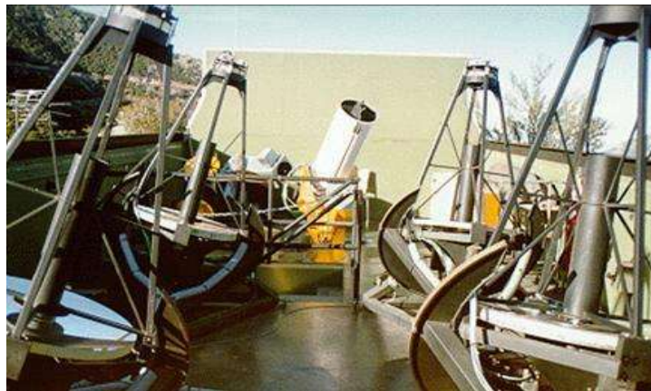
The three original robotic telescopes at the rear of the Fairborn Observatory are almost obscured by the four 0.8-meter telescopes that were subsequently added—completely filling up the available space. These seven robotic telescopes observed together harmoniously every clear night on Mt. Hopkins for many years.
