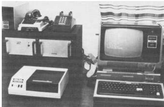
Russ Jr. (1979) centers a star at the Fairborn Observatory's first telescope (left). The UBV photometer, DC amplifier, high voltage power supply, and strip chart recorder are visible. A Radio Shack TRS-80 microcomputer (right) was used for data reduction. Also shown are a thermal printer, modem, and (upper left) a floppy drive.
