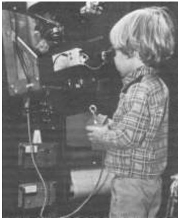
Russ Jr. (1979) centers a star at the Fairborn Observatory's first telescope (left). The UBV photometer, DC amplifier, high voltage power supply, and strip chart recorder are visible. A Radio Shack TRS-80 microcomputer (right) was used for data reduction. Also shown are a thermal printer, modem, and (upper left) a floppy drive.
