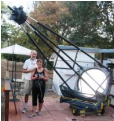
Russ and his wife Cheryl, a philosophy professor, stand beside Russ’ 1-meter portable telescope. For transport, the telescope, with its top truss structure disassembled, fits into the back of a Jeep Cherokee.
